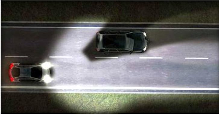
The BeamAtic lighting automation system takes over the lighting commands to optimize the use of high beam. It switches back to low beam as soon as an oncoming or leading car is detected by the embedded camera. The system alleviates the stress of constantly switching the headlamps on and off, thus improving night-time driving comfort and safety.
